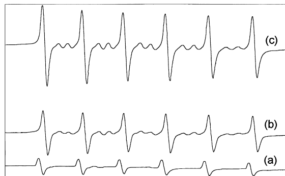
Fig. 3. ESR spectra of \text{Mn}^{3+}/\text{MgO} (pure) after hydrogen spillover at 653 K from Pt/ \text{SiO}_2 for: (a) 4 h; (b) 24 h; (c) 48 h.
